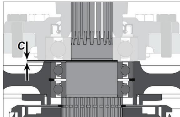
(34) Measure distance “C” between the output shaft and bearing thrust block.
