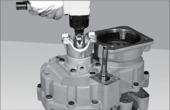
(3) Remove the nut (1) and O-ring (2) and pull out the flange (3).
