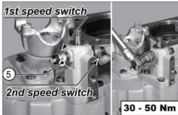
(14) Engage the 1st speed and verify with a control device (tester) that the switch 1st speed gives signal and that the switch 2nd speed is disabled.
