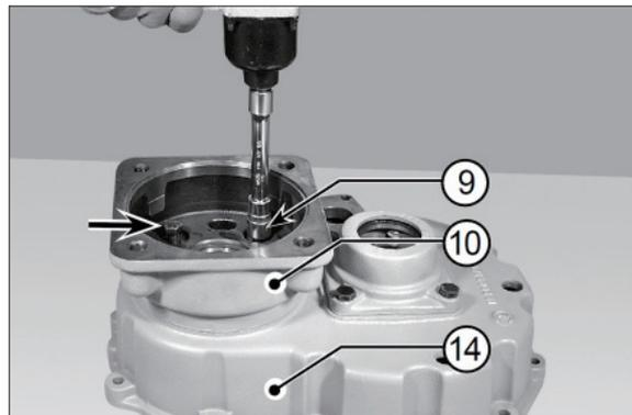
(29) Remove the cover by fixing the distance washers (12) onto the cover (10) itself.
