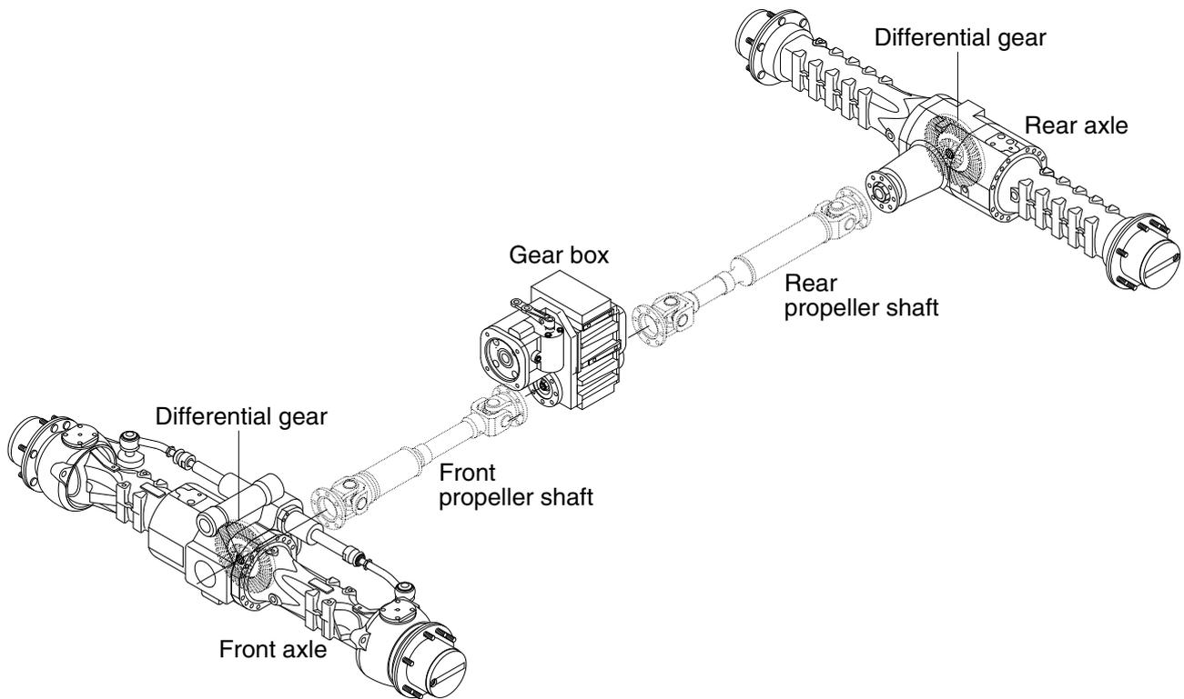
The differential is installed on the front and rear axle to transfer the driving torque from the axle to the wheels. The differential transfers half of the output torque of the transmission via the universal drive shaft to the planetary gear of the wheel hubs and transfers the rpm and torque from the gear via the pinion and the ring.
