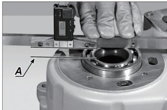
(9) Calculate thickness “S” of the shims by using this formula :
