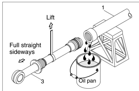
Note that the plated surface of rod assembly (3) is to be lifted. For this reason, do not use a wire sling and others that may damage it, but use a strong cloth belt or a rope.
