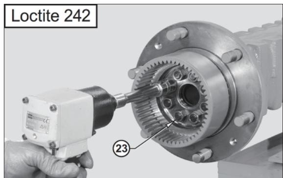
⑫ Tighten nuts (23) in two stages, using the criss-cross method.
