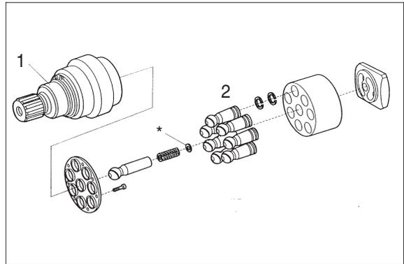
(1) Remove fixing screw (cylinder).
