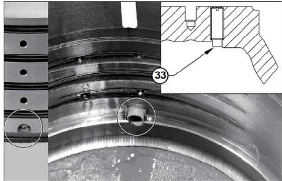
②④ Insert the brake module facing the input holes to the top.
