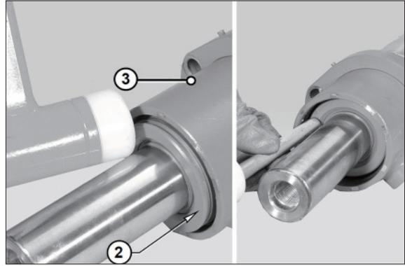
⑨ Using a punch, force the stop ring (4) located inside the cylinder (3) and extract ring using a screwdriver.
