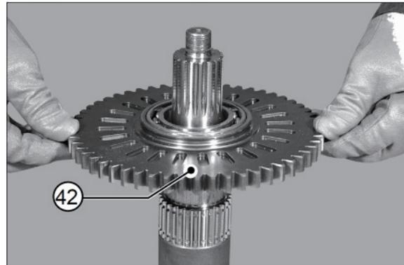
(25) Remove the bearings (21) from the gear (42).
