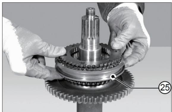
(18) Secure the synchroniser (25) in position with the snap ring (26).
