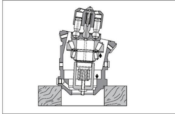
(6) Fix zero position of cylinder with  $Q_{max}$  screw.
