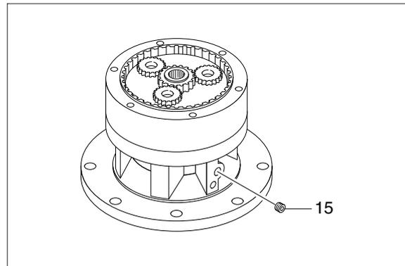
(8) Mount No.2 carrier assembly (12) in the case sub assembly and install bolts into 2 TAP holes (M6) as shown in figure.
