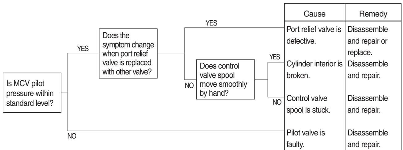
6) BOOM MAKES A SQUARING NOISE WHEN BOOM IS OPERATED
