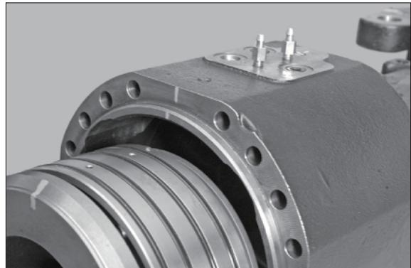
②⑤ Insert the piston to the end stop by alternating light strokes and remove the screws.
