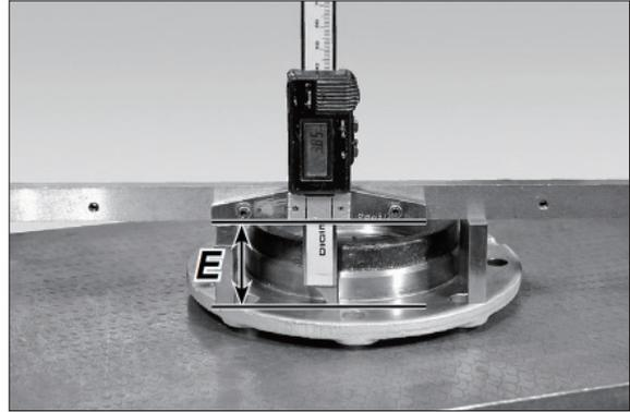
(41) Calculate thickness "S4" of the shims by using this formula :
