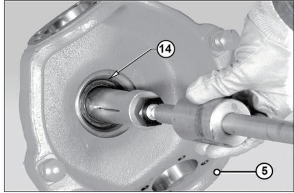
②⑥ Remove the bushing (6) from the steering case (14).
