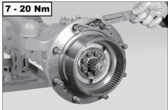
※ Check the condition and position of the O-ring (37).
