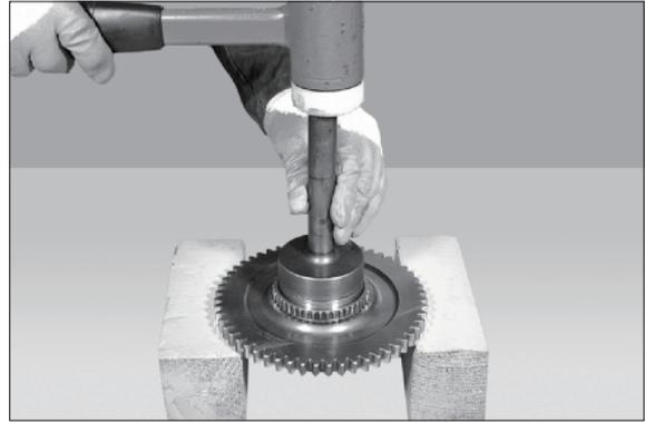
(15) Fit gear (42) onto the shaft (24).
