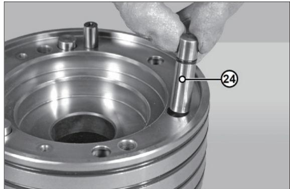
④ Remove the O-rings and the anti-extrusions rings from the service brake, the negative brake piston and from the piston.
