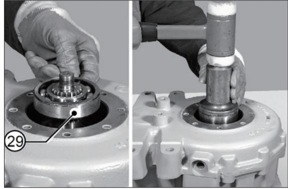
(37) Re-insert the new sealing ring (31) in the motion output cover (41).
