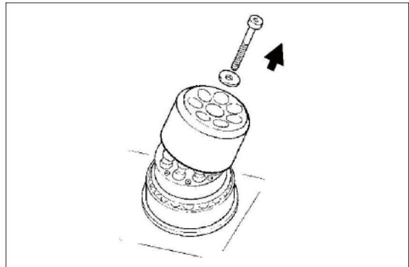
(2) Disassemble retaining plate.
