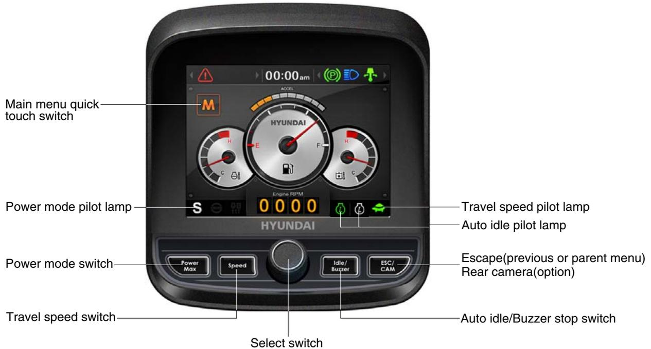
※ When the switches are selected, the pilot lamps are displayed on the LCD. Refer to the page 4-11 for details.
