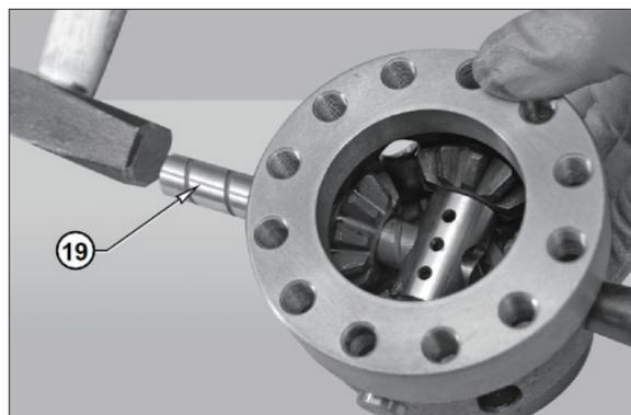
⑥ Center the pin holes and insert the 3V pins (20).
