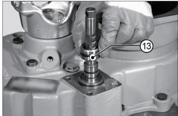
(9) Remove the snap ring (12) securing the piston (13).
