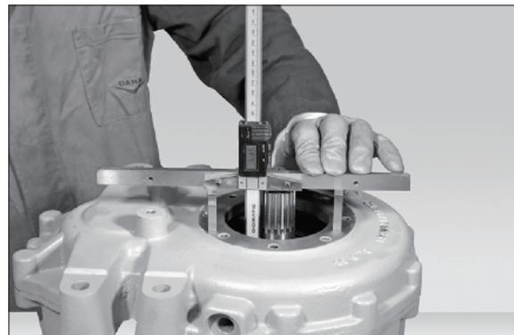
(35) Calculate thickness “S3” of the shims by using this formula :
