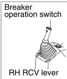
(1) On pressing this switch, the breaker operates only when the breaker selection switch on the switch panel is selected.
