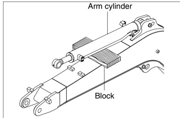
② Remove bolt (2) and pull out pin (1).
