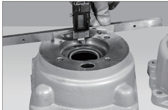
(8) Measure distance “A” between the surface and thrust block.
