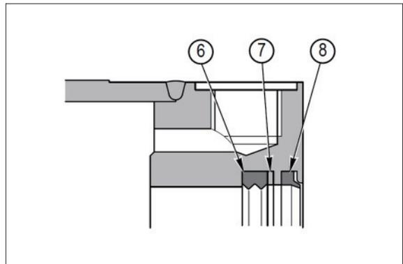
② Grease and install the piston rod seal ring (6), rod wiper (8) and anti-extrusion ring (7) into the head (2).
