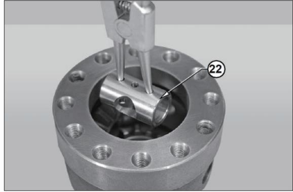
⑳ Remove the planetary gear (16).
