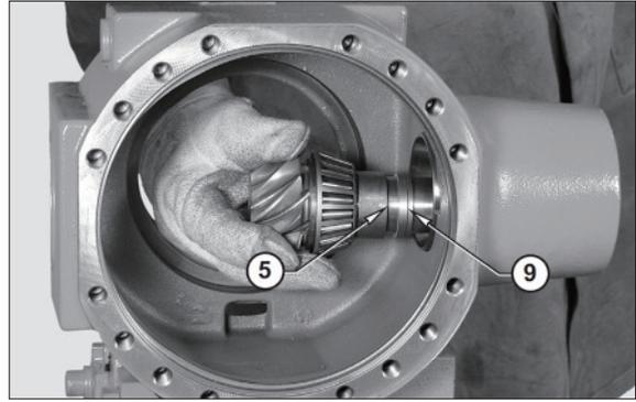
⑭ Heat the external bearing (14) to a temperature of about 100°C and fit it on to the pinion (11) so as to complete the pack as shown in the figure.
