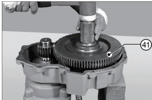
(25) By hand install the bearing on the input shaft.
