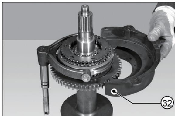
(21) Secure the lower shaft assembly (24) to a hoist.
