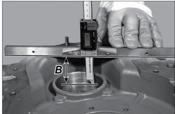
(28) Calculate thickness “S2” of the shims by using this formula :
