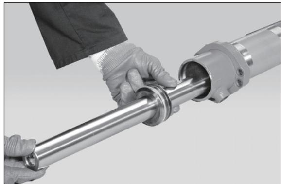
① Remove all seals, anti-extrusion rings and scraper rings from head (2), cylinder (3) and piston (5).
