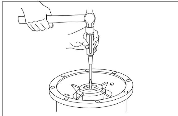
**(16) Disassembly of cylinder assembly**
