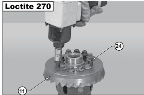
⑪ Tighten screws with a torque wrench : see table.
