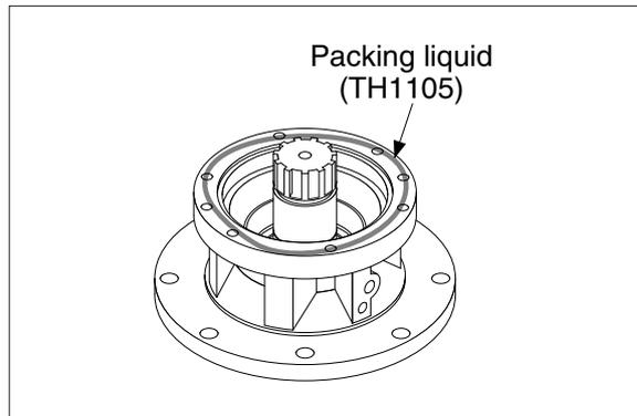
(5) Place ring gear on the case by matching it with knock pin hole.
