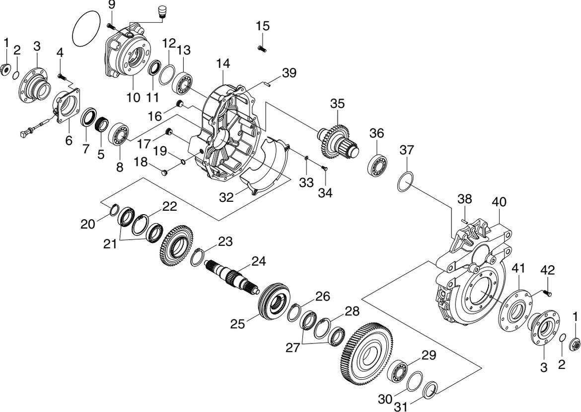
(1) Remove the gear control cylinder.
