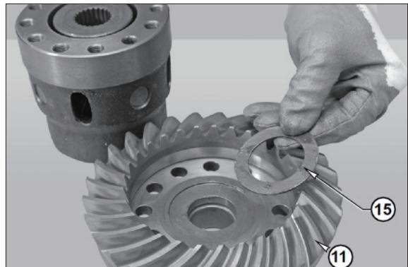
⑩ Position the crown (11) on the differential carrier and lock it with screws (24) applied with loctite 270.
