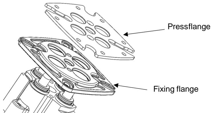
8) Disassembly the pilot curve kits the four kits is the same composition
