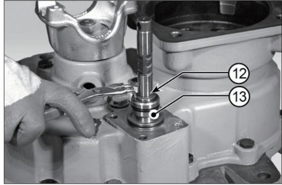
(8) Remove the piston (13), complete with seals.
