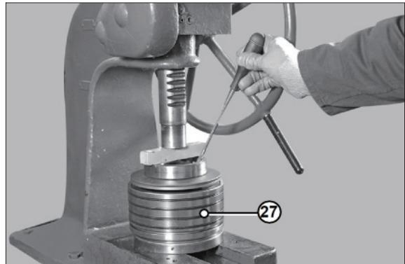
⑳ Screw down the slotted nut to the earlier determined position.
