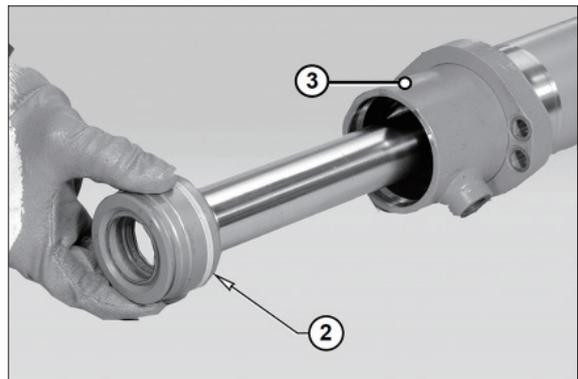
※ Note down direction of installation of piston whose seal ring is oriented towards cylinder head.
