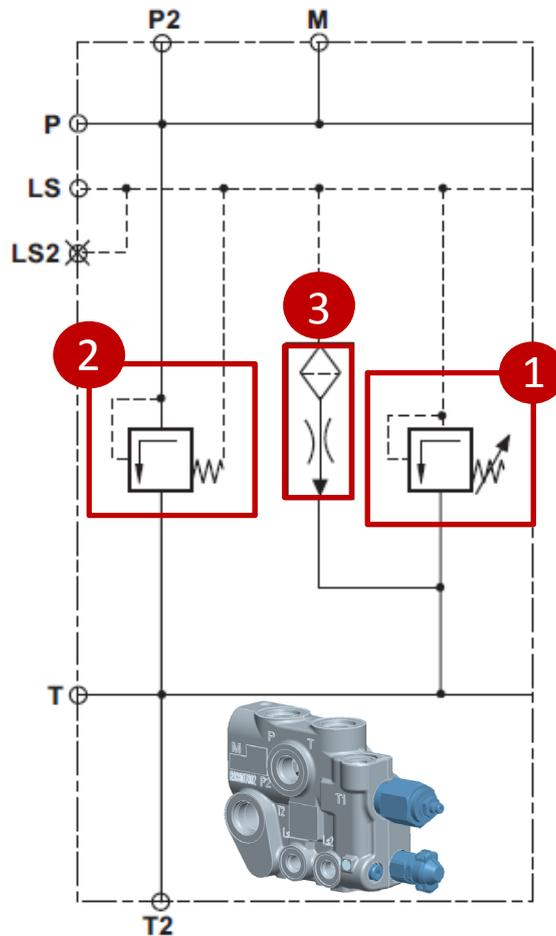
1. LS relief valve: overflow LS oil line working pressure
