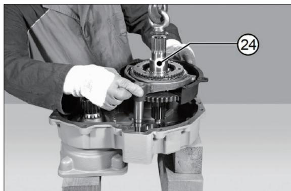
(22) Using a plastic hammer, install the lower shaft (24).
