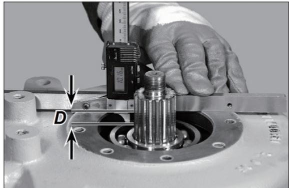
(39) Zero the depth gauge between calibrated blocks (whose known thickness is 30 mm) and bearing seat.
