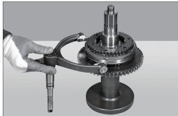
(21) Remove the snap ring (26) securing the synchroniser (25).
