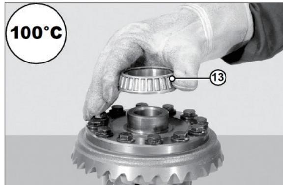
⑬ If the bearings are replaced, insert the external thrust blocks in the middle cover and in the central body.
