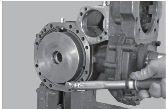
⑯ Check that the positioning of the sealing ring on the arm is intact; install the complete arm. Lock it into position using two facing screws and washers.
