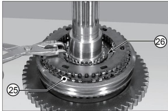
(19) Fit the gear selector yoke in the synchroniser (25).
