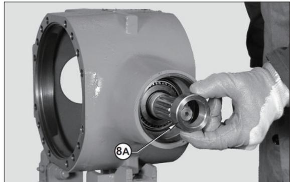
⑯ Install the flange (2) onto the pinion (11) without sealing ring.
