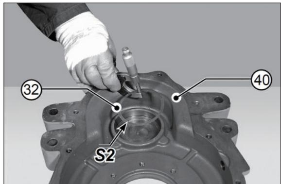
(29) Using a normal tool, push the bearing (36) and shims into its seat in the cover (40).
