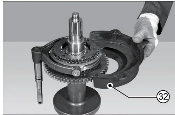
(20) Remove yoke and gearbox control rod.
