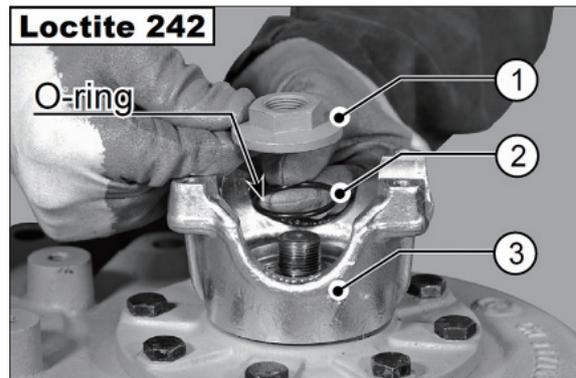
(46) Tighten the lock nut (1) to a torque of 28.6~31.6 kgf · m (207~229 lbf · ft).
