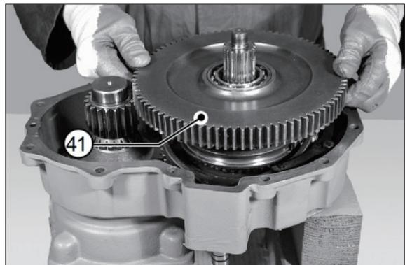
(14) Remove the bearing (27) from the gear (41).
