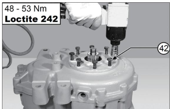
(44) Fit the flange (3) on the shaft (24), seating completely.
