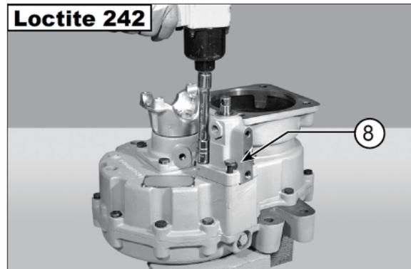
(9) Tighten screws (8) using a torque wrench setting of 4.89~5.4 kgf · m (35.4~39.1 lbf · ft).
