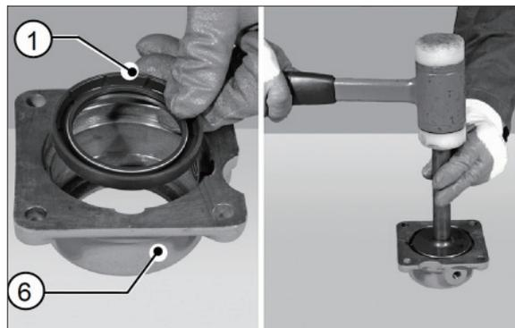
(2) Using a normal tool insert the bearing (8).
