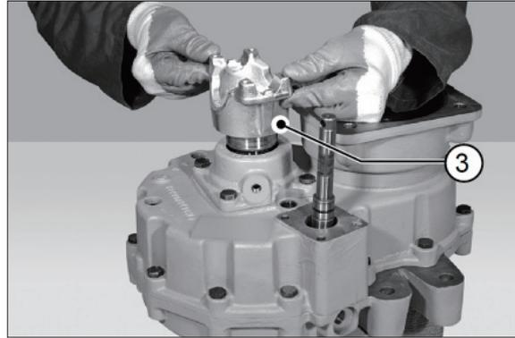
(49) Lubricate the O-ring (2) with grease and fit in the flange (3) seating. Spread with loctite 242 the lock nut (1) and fit.
