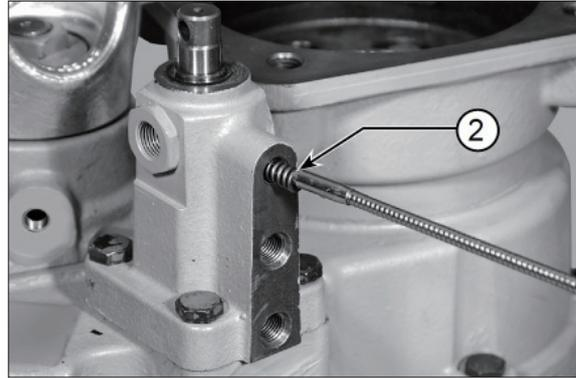
(12) Coat the dowel (1) with loctite 510 and screw it until it is level with the cylinder.
