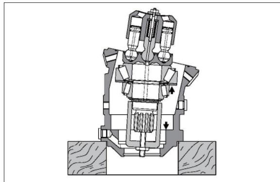
(5) Insert rotary group into housing to seat position.
