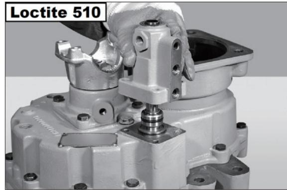
(8) Assembly the screws (8), spreading loctite 242 on screws.
