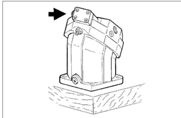
(7) Assemble shaft seal, disc and safety ring.
