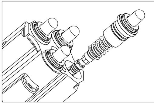
9) Disassembly the curve kits, the seal will not be separated to repair, and it need to replacèd with piston together as the relative parts list
