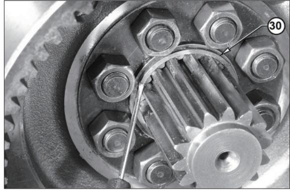
⑦ Unloose and remove the tightening nuts (32) from the crown flange (35).
