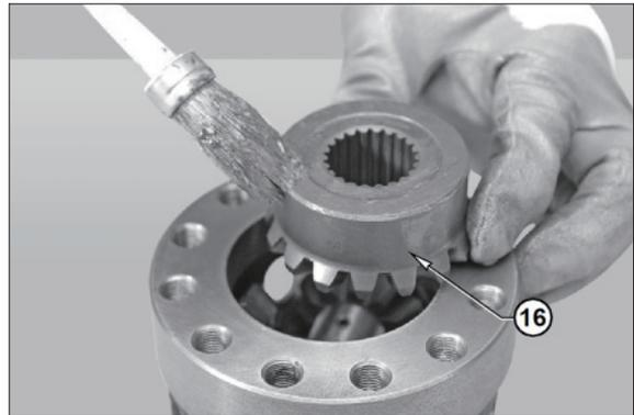
⑧ Insert planetary gear wheel (16).
