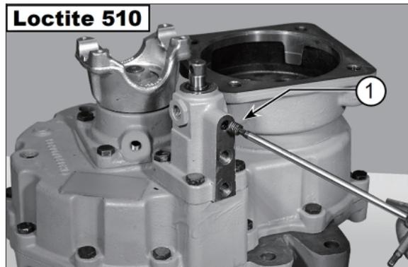
(13) Fix the gear-in position switch (4) with washer (7) and O-ring (5), (6).
