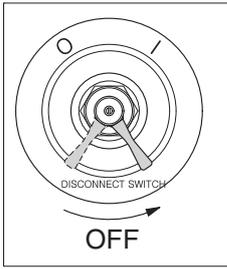
(1) This switch is used to shut off the entire electrical system.
