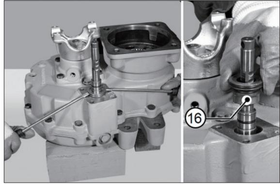
(12) Remove the dust scraper ring (10) and the rod's O-ring (11) from the gearshift cylinder (9).
