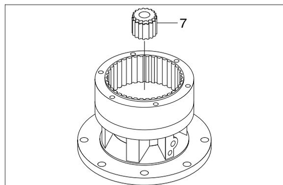
(10) Mount No.1 carrier assembly (10) in the case sub assembly and install bolts into 2 TAP holes (M6) as shown in figure.
