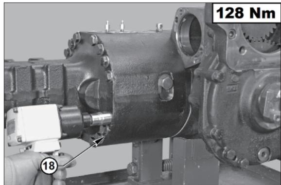
(13) Check the flatness of the arms; then lock the arms into their final position, using screws adequately coated with loctite 242.
