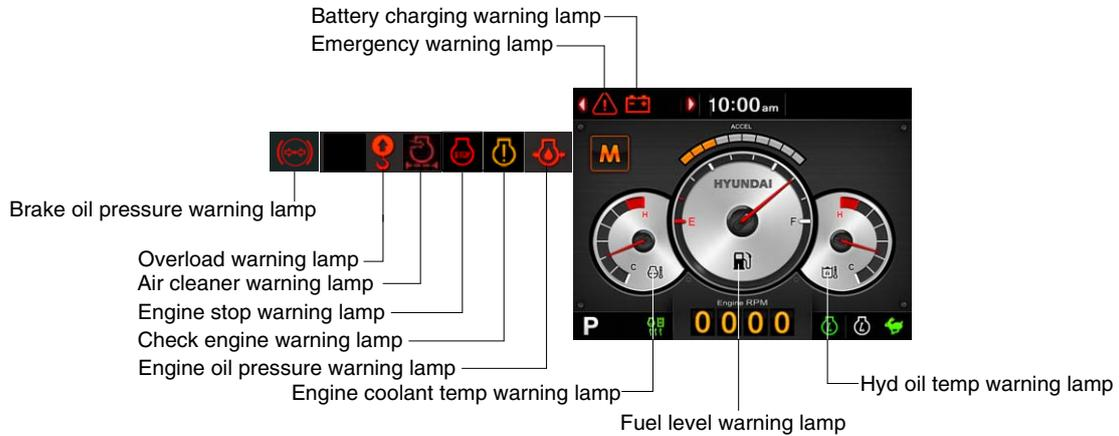
※ Each warning lamp on the left-top of the LCD pops up on the center of LCD and the buzzer sounds when the each warning is happened. The pop-up warning lamp moves to the original position and lights ON when the buzzer stop switch is pushed or the pop-up is touched. And the buzzer stops. Refer to page 4-14 for the switch.
