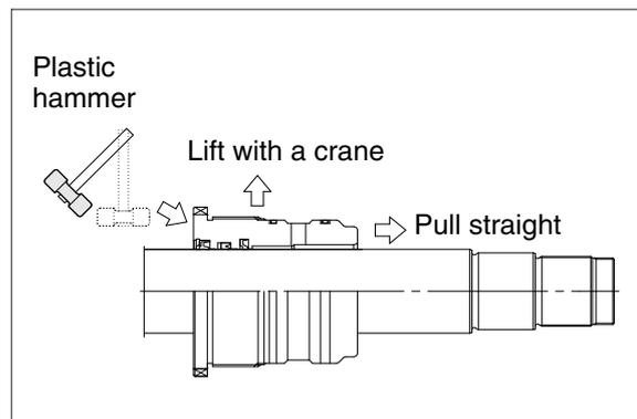
**(3) Disassemble the piston assembly**
