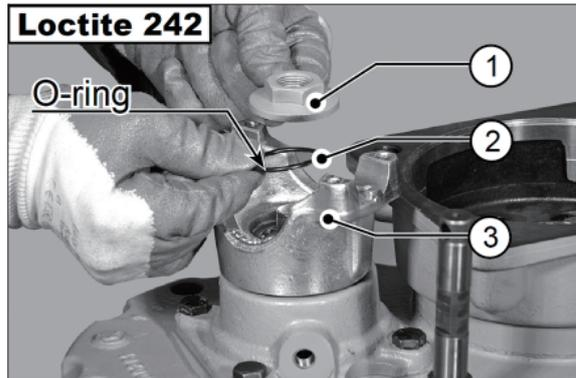
(50) Tighten the lock nut (1) to a torque of 28.6~31.6 kgf · m (207~229 lbf · ft).
