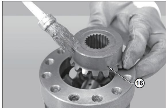
⑧ Insert planetary gear wheel (16).
