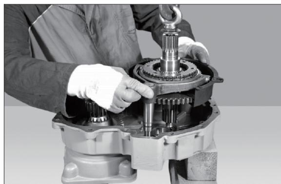
(19) Remove the internal baffle plate (32).
