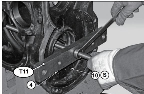
※ Before starting the next stage, make sure that the thrust block has been completely inserted into its seat.
