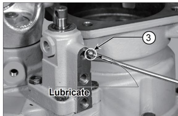
(11) Fit the gear selector springs.
