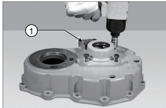
(33) Disjoin and remove the cover (6).
